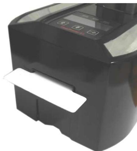
*Picture 5: Cleaning card in cleaning position*
