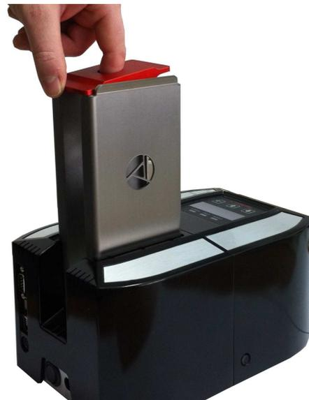
*Picture 2: Insert "Hopper Load"*
